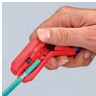
Stripping of a data cable
