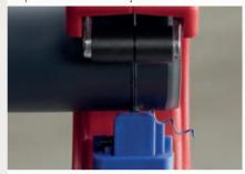
Segments as short as 10 mm can be cut. The spiral chip comes from chamfering.
