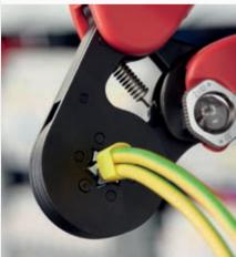
Also suitable for twin wire ferrules: capacity up to 2 x 10 mm<sup>2</sup>
