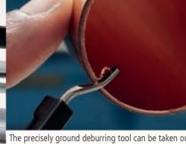
The precisely ground deburring tool can be taken out of the tool when needed.
