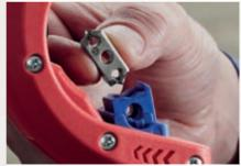
When worn, the blade can be reversed or replaced without the need for tools.
